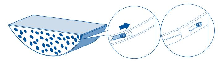
When putting on the cover, pull on the cover with one hand and push the foam piece with the other. This helps when replacing the cover.
